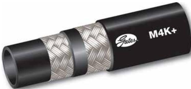
**Braided reinforcement can be made of wire or textile, and can have one or multiple layers. It is light-weight and flexible for medium and low-pressure hose applications.**
