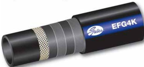
**Spiraled reinforcement is typically wire and has four or six layers (plies). It is designed to handle more severe applications with longer impulse service life.**
