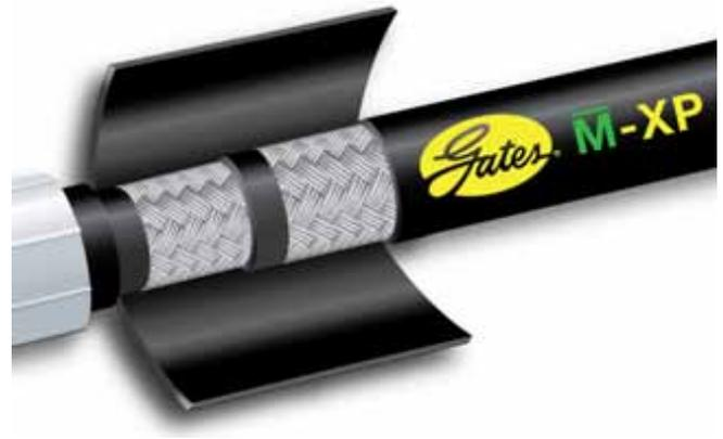
M-XP hose has been tested at an industry-leading 1,000,000 impulse cycles (at 212°F; 100°C), which exceeds the SAE standard of 200,000 impulse cycles and the Gates minimum requirement of 600,000 impulse cycles for typical wire-braid hoses. The high-impulse cycle testing increases service life and makes M-XP hose ideal for out-of-sight and hard-to-reach applications such as boom arms and scissor lifts used in the mobile equipment and construction markets.
